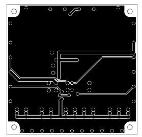
L2 : Copper wiring pattern diagram
