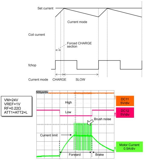
The limit current is set as calculated on the basis of the voltage input to the VREF pin and the resistance between the RF pin and GND using the formula given below.
