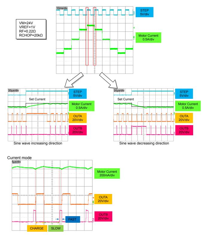
When the motor current reaches to the setting current, it is switched to Slow Decay mode. Motor current switches from Slow Decay mode to Fast Decay mode for 1/16 of one chopping cycle.
