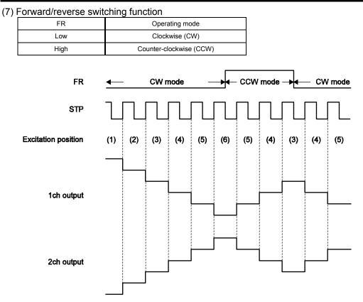
The internal D/A converter proceeds by one bit at the rising edge of the input STEP pulse. In addition, CW and CCW mode are switched by setting the FR pin. In CW mode, the channel 2 current phase is delayed by 90° relative to the channel 1 current. In CCW mode, the channel 2 current phase is advanced by 90° relative to the channel 1 current.
