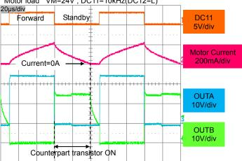
(synchronous rectification) . After motor current fades off, output turns off. Synchronous rectification reduces heat generation compared to diode regeneration.
