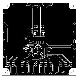
L1 : Copper wiring pattern diagram
