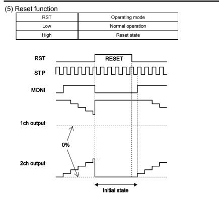
When the RST pin is set to High, the excitation position of the output is forcibly set to the initial state, and the MONI output is placed in the ON state. When RST is then set to Low, the excitation position is advanced by the next STEP input.
