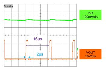
(7) Typical current waveform in each excitation mode when stepping motor parallel input control
