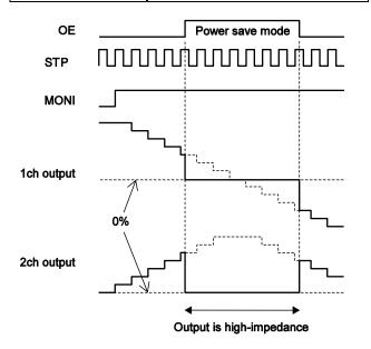
When the OE pin is set High, the output is forced OFF and goes to high impedance. However, the internal logic circuits are operating, so the excitation position proceeds when the STEP signal is input to the STP pin. Therefore, when OE is returned to Low, the output level conforms to the excitation position proceeded by the STEP input.
