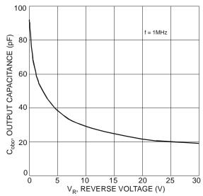
Figure 6 Typical Output Capacitance Characteristics
