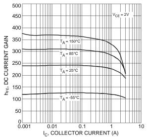
Figure 2 Typical DC Current Gain vs. Collector Current
