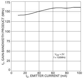
Figure 7 Typical Gain-Bandwidth Product vs. Emitter Current
